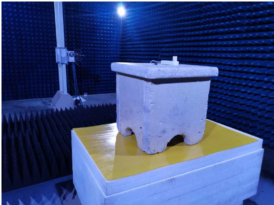
Photo of Radiated Emission Measurement Above 1GHz
