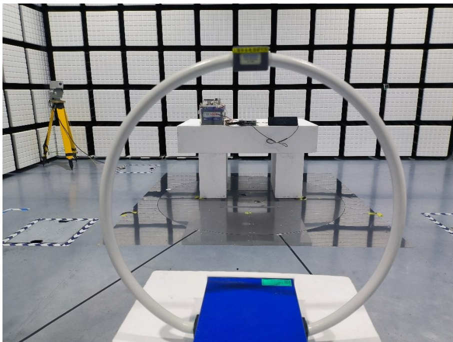
Description: Radiated Emission Test Setup (Below 30MHz)
