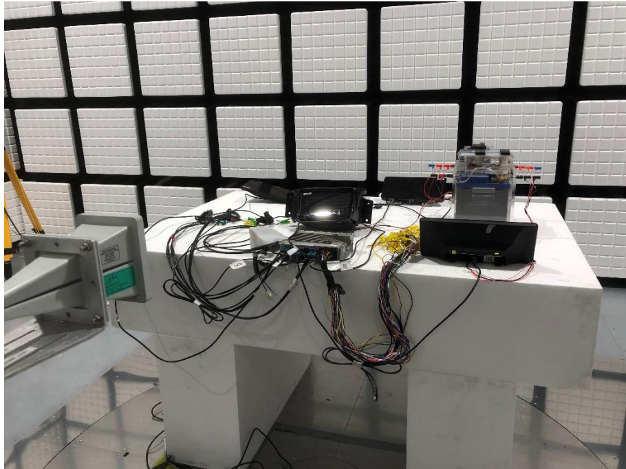
Description: Radiated Emission Test Setup (Above 18GHz)
