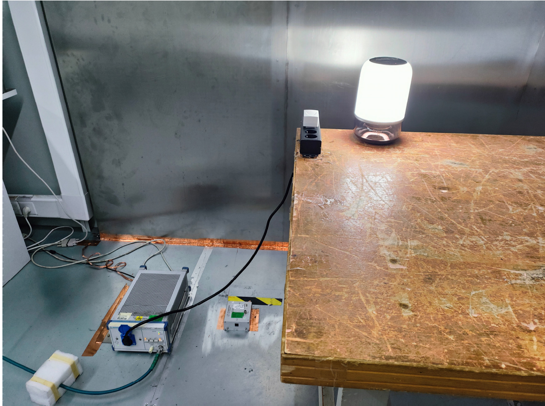
Conducted Emissions - Side View
