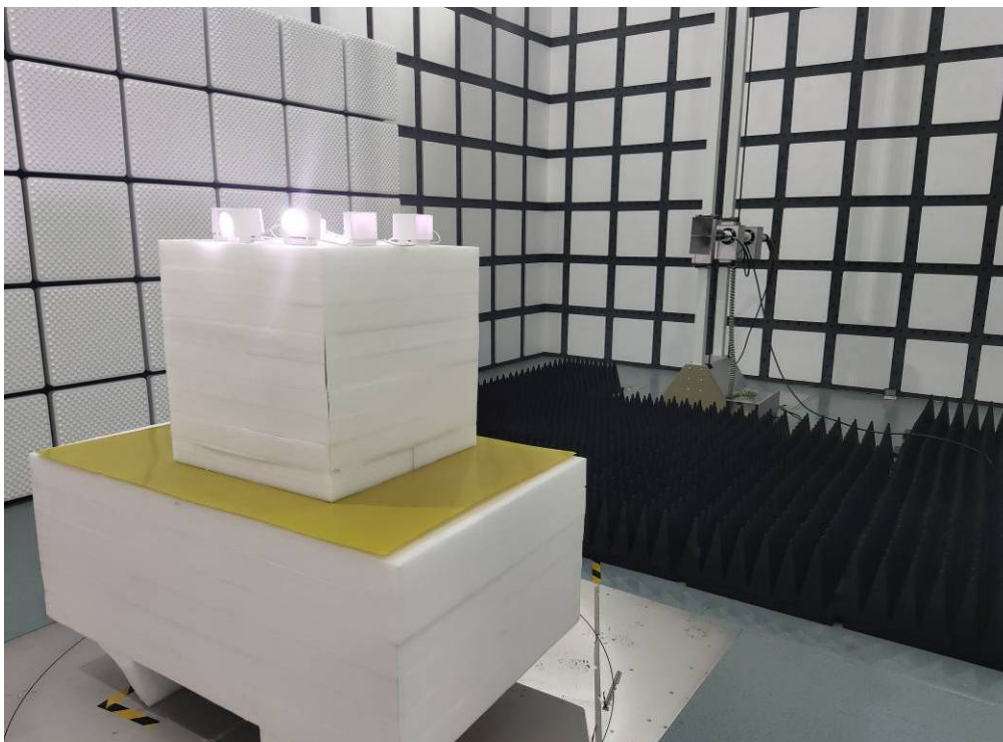
Photo of Radiated Emission Measurement (Above 1G)
