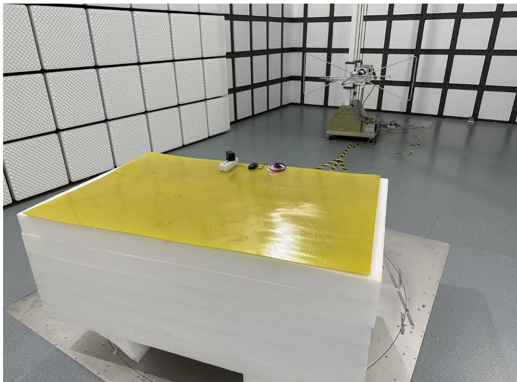
Photo of Radiated Emission Measurement (Above 1G)
