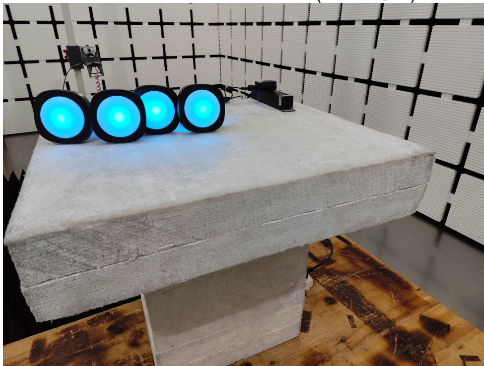
Photo of Radiation Emission Test (above 1GHz)
