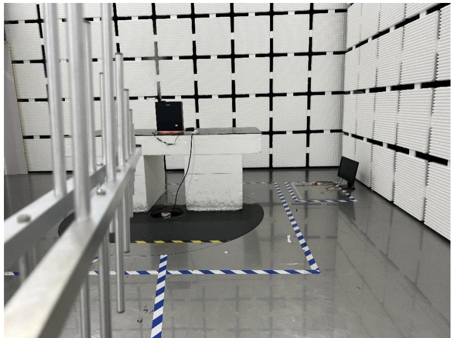
Radiation Emission Test Setup (30MHz to 1GHz)
