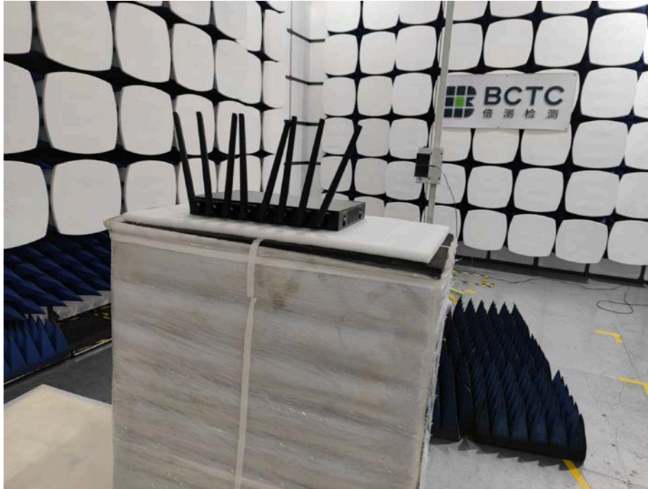
Spurious Emission Test Setup (Above 1GHz)
