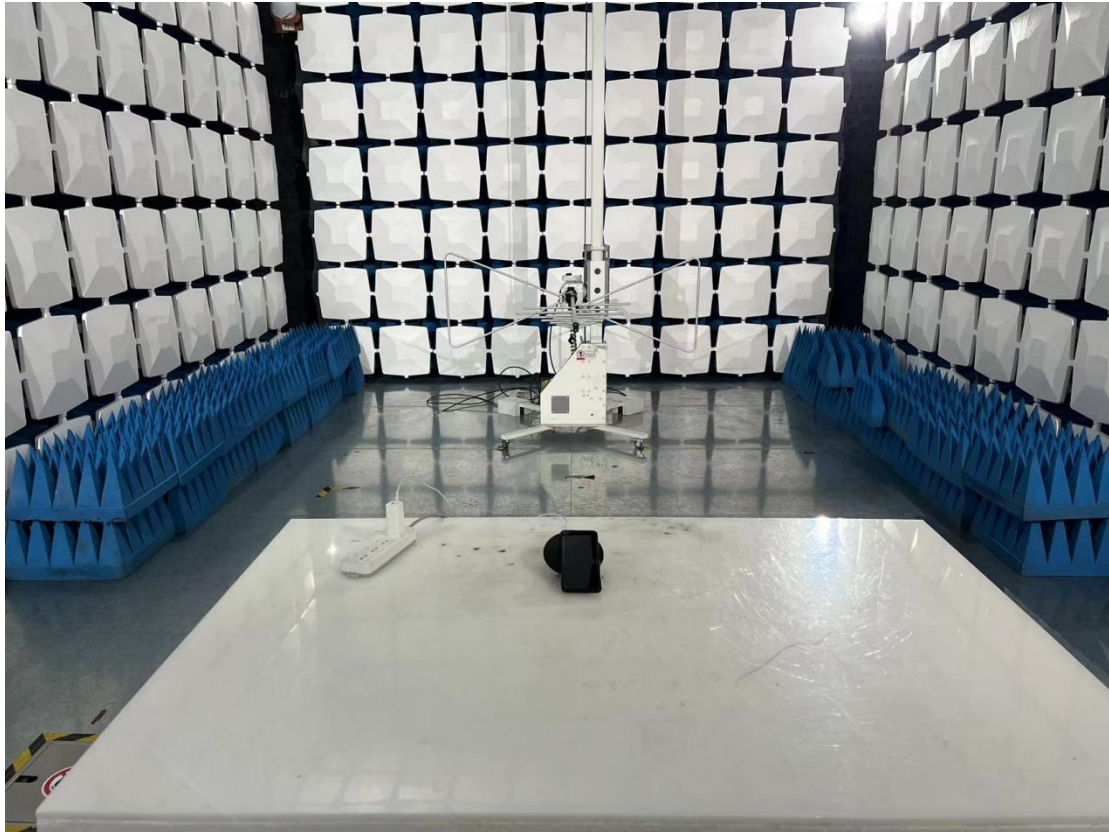
Blow 1GHz for radiated emission test setup
