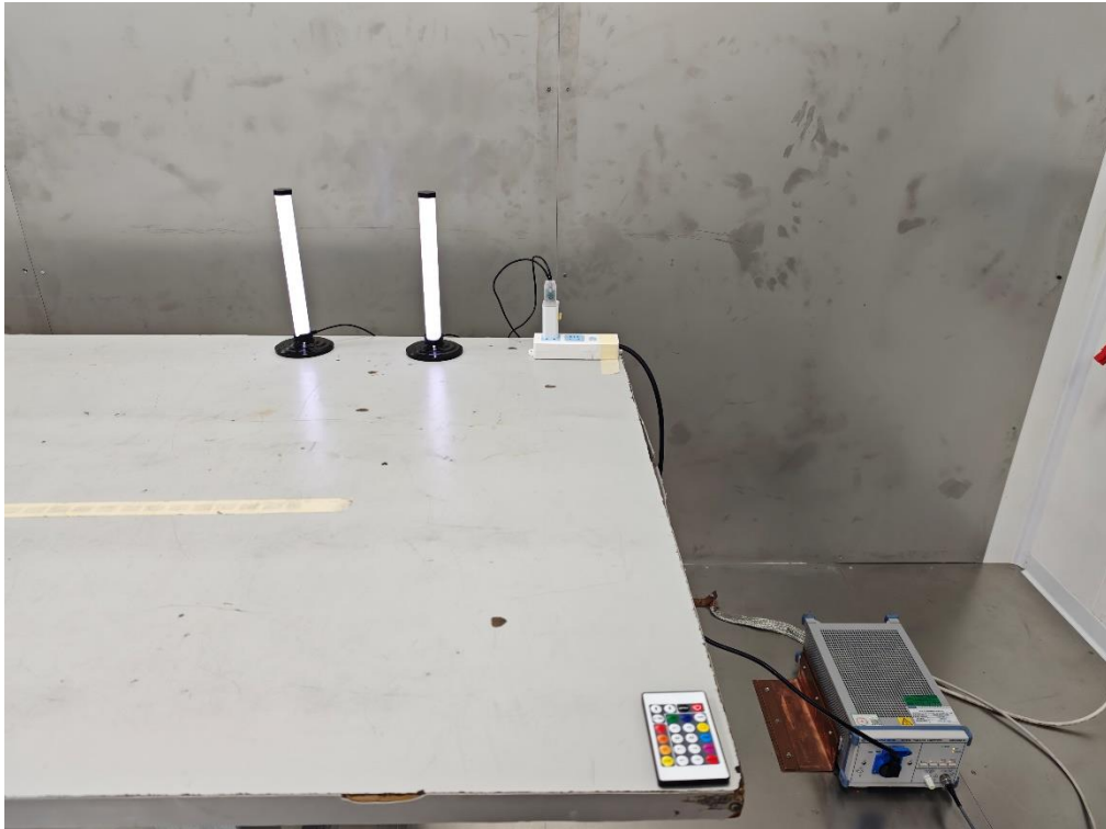
AC Conducted Measurement Photos
