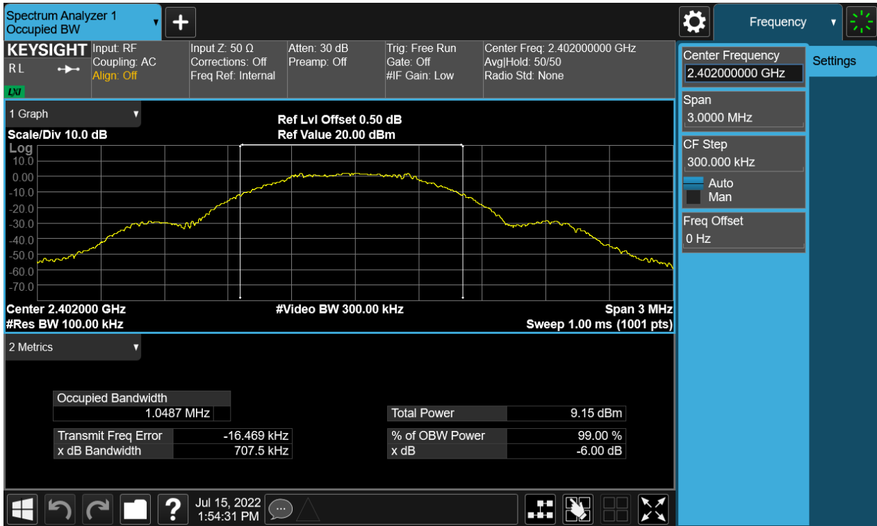
Figure 8: 6dB Bandwidth, BLE_1Mbps_2440MHz
