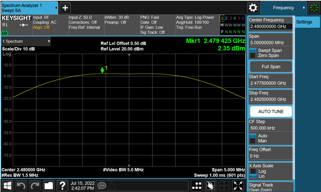
Figure 6: Peak Output Power, BLE_2Mbps_2480MHz
