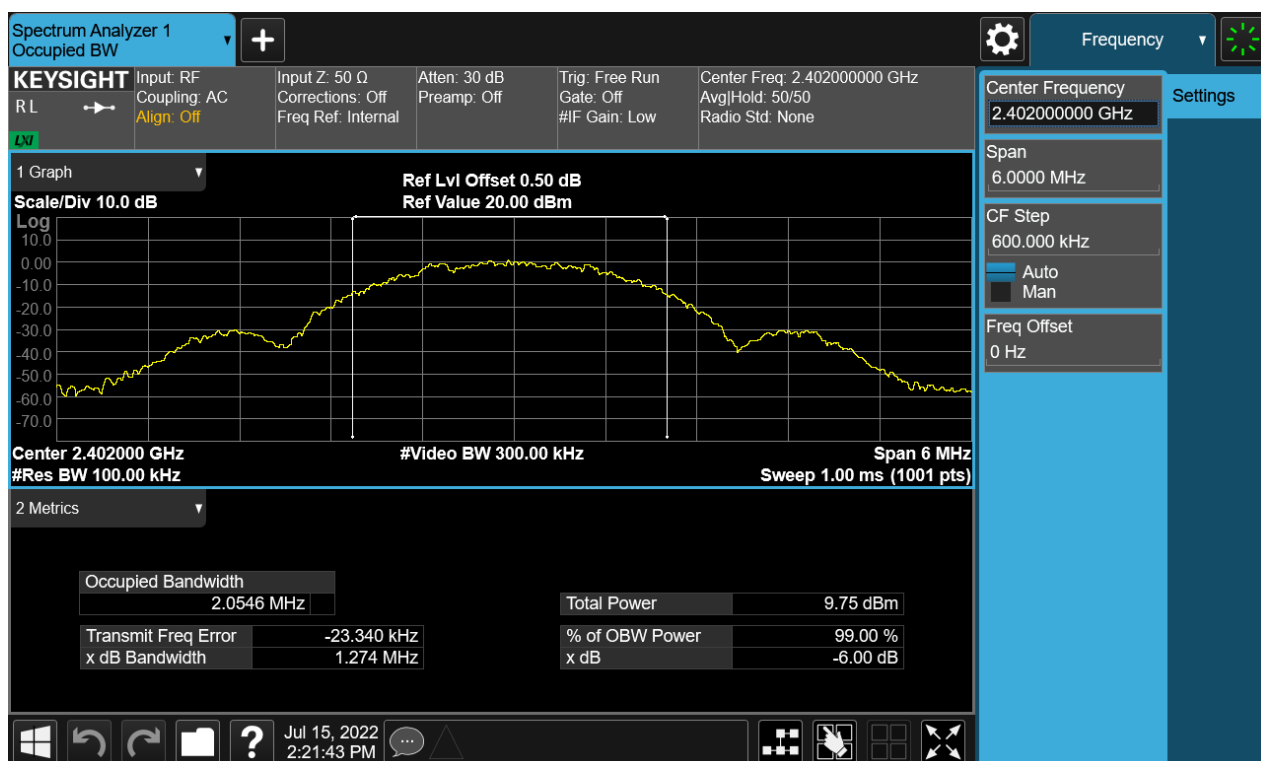
Figure 10: 6dB Bandwidth, BLE_2Mbps_2402MHz
