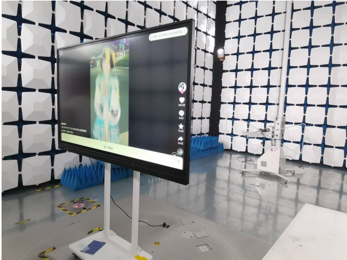
Above 1GHz for radiated emission test setup
