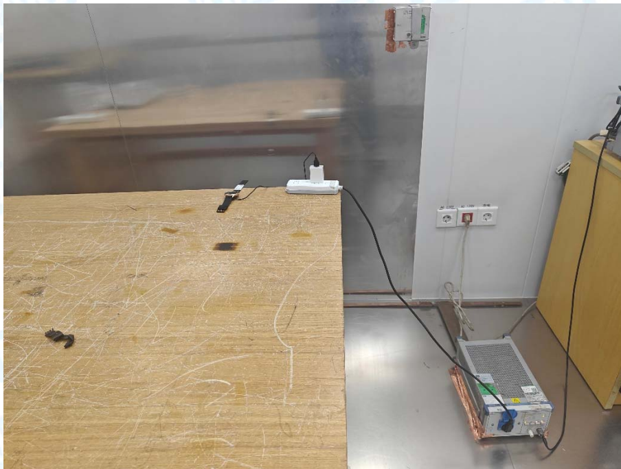
Photo of Setup for Conducted Emission
