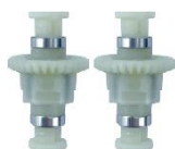
Differential gearbox in both of front and rear
