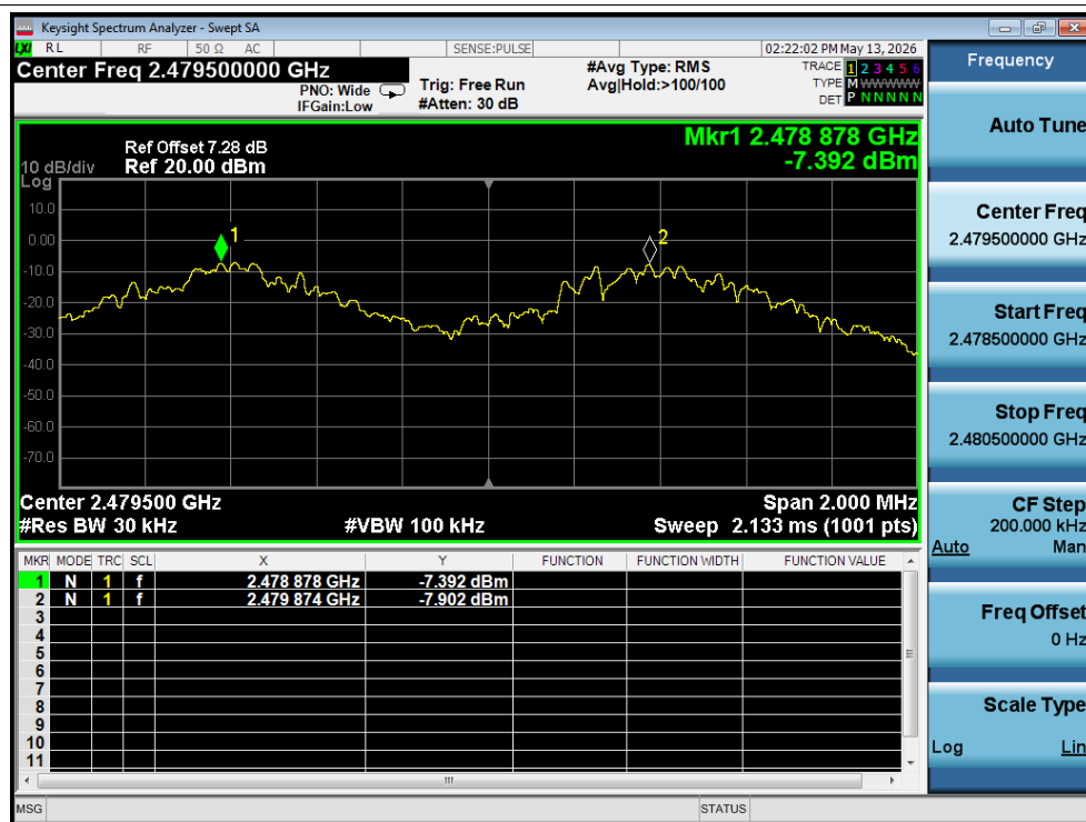
CFS NVNT 1-DH5 2480MHz Ant1
