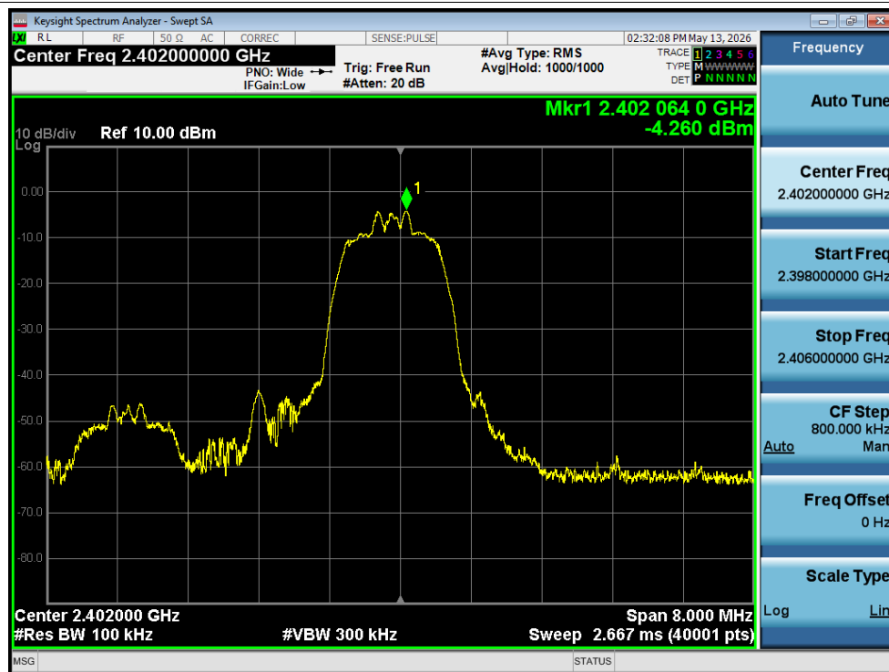
Tx. Spurious NVNT 2-DH5 2402MHz Ant1 Ref
