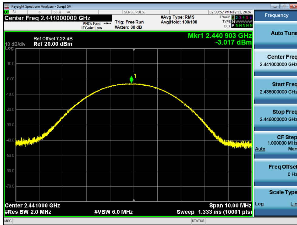
Peak Power NVNT 2-DH5 2441MHz Ant1
