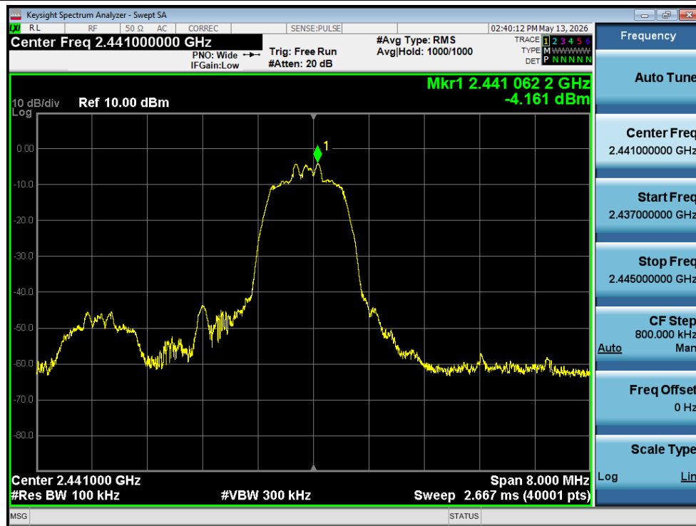
Tx. Spurious NVNT 2-DH5 2441MHz Ant1 Ref
