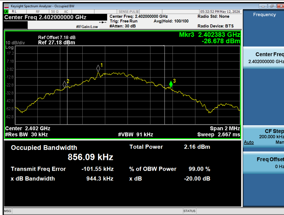
-20dB Bandwidth NVNT 1-DH5 2402MHz Ant1
