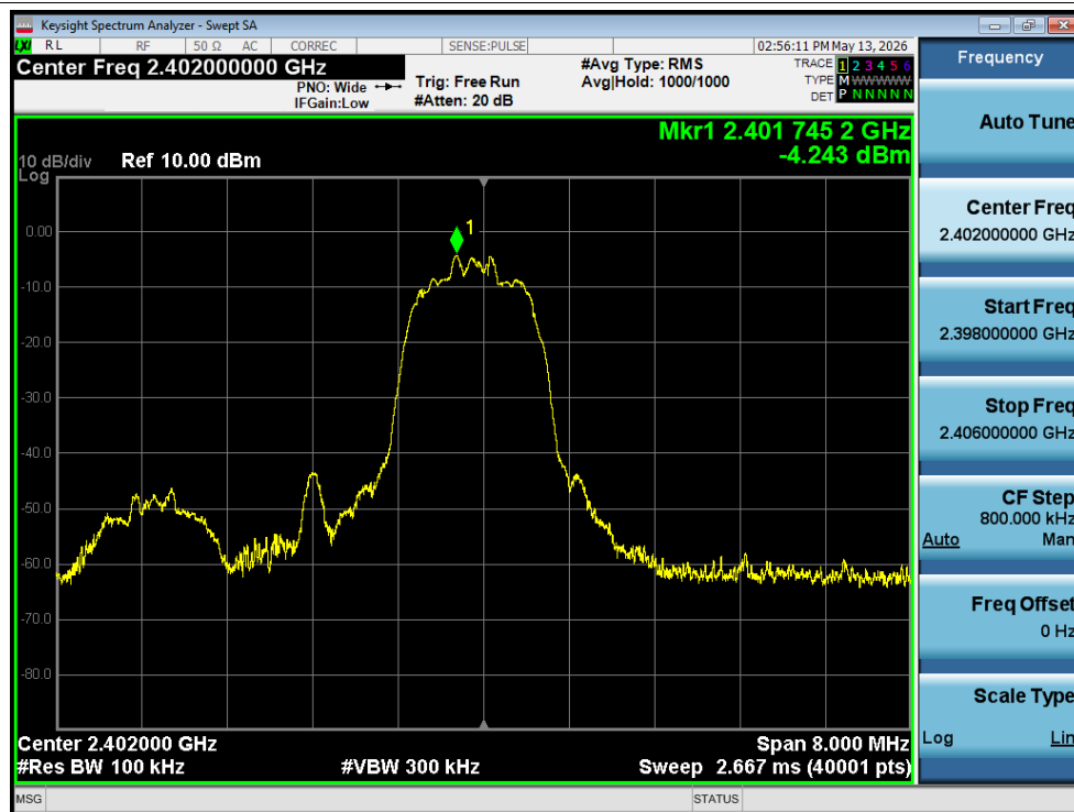
Tx. Spurious NVNT 3-DH5 2402MHz Ant1 Ref
