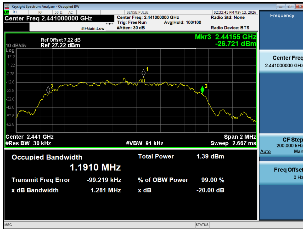
-20dB Bandwidth NVNT 2-DH5 2441MHz Ant1
