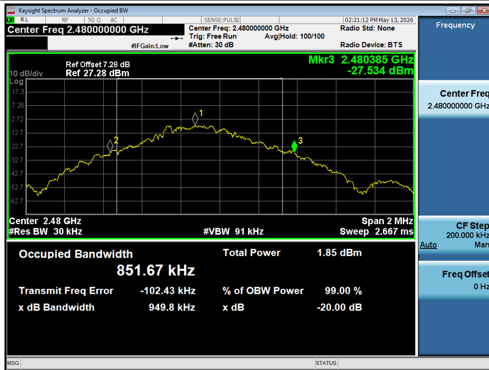
-20dB Bandwidth NVNT 1-DH5 2480MHz Ant1
