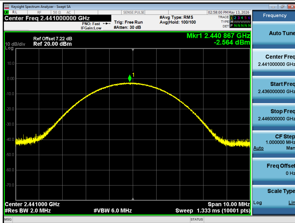
Peak Power NVNT 3-DH5 2441MHz Ant1
