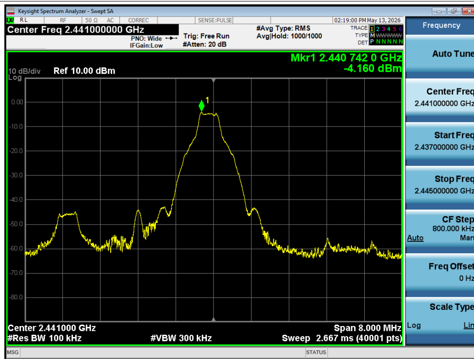
Tx. Spurious NVNT 1-DH5 2441MHz Ant1 Ref
