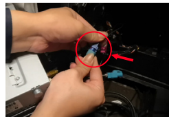
8. Connect original car LVDS cable with carplay box LVDS cable
