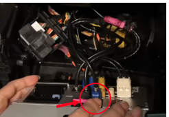
7. Unplug the LVDS cable from multimedia box (most time is a blue head)
