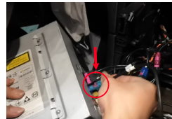
9. Plug the CarPlay LVDS cable to the multimedia box.
