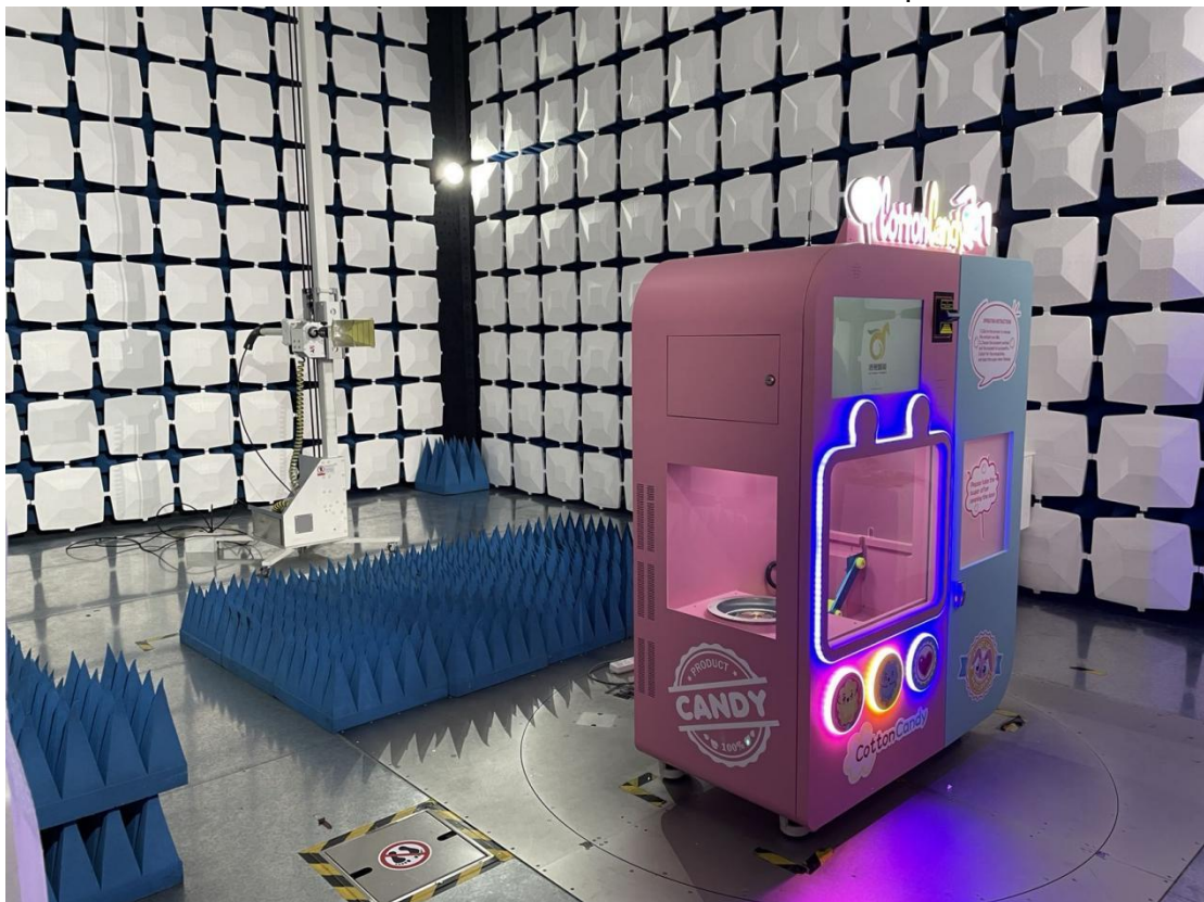
Above 1GHz for radiated emission test setup
