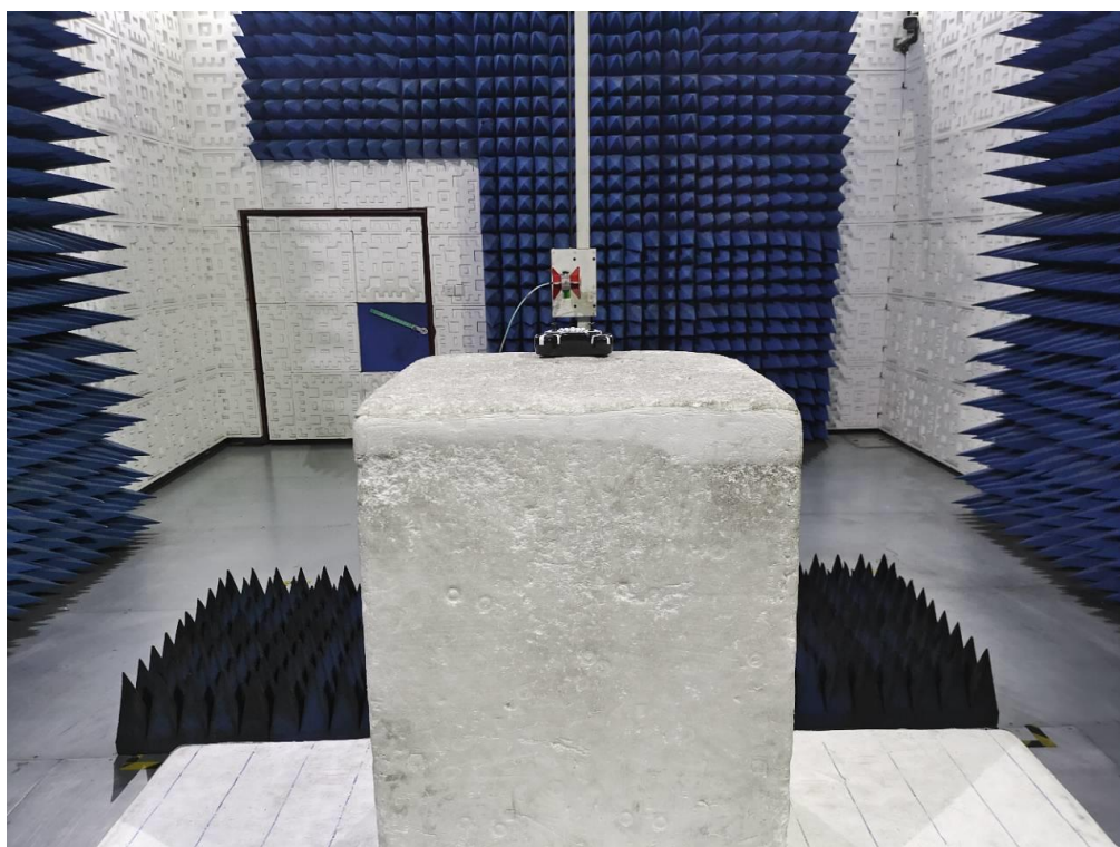
RADIATED EMISSION TEST SETUP ABOVE 1GHz
