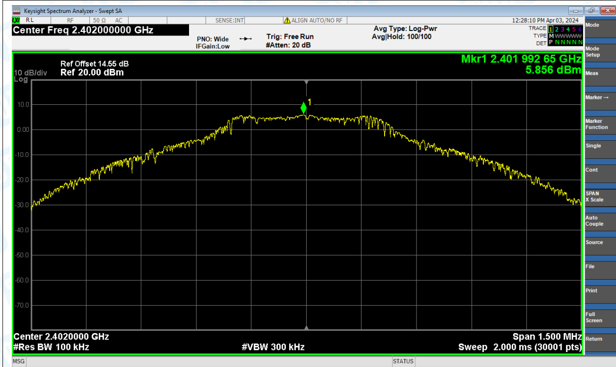
Tx. Spurious NVNT 1-DH1 2402MHz Ant1 Emission
