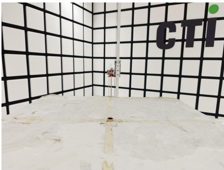
Radiated spurious emission Test Setup-2(Above 1GHz)
