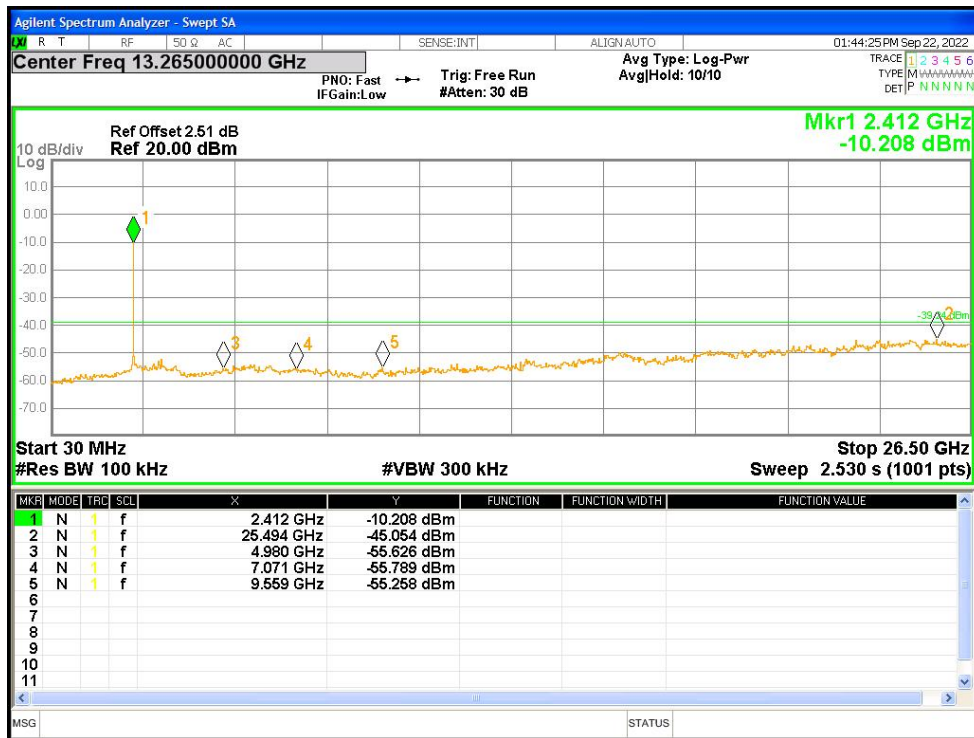
Tx. Spurious NVNT g 2437MHz Ant1 Ref
