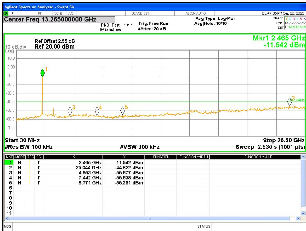
Tx. Spurious NVNT n20 2412MHz Ant1 Ref
