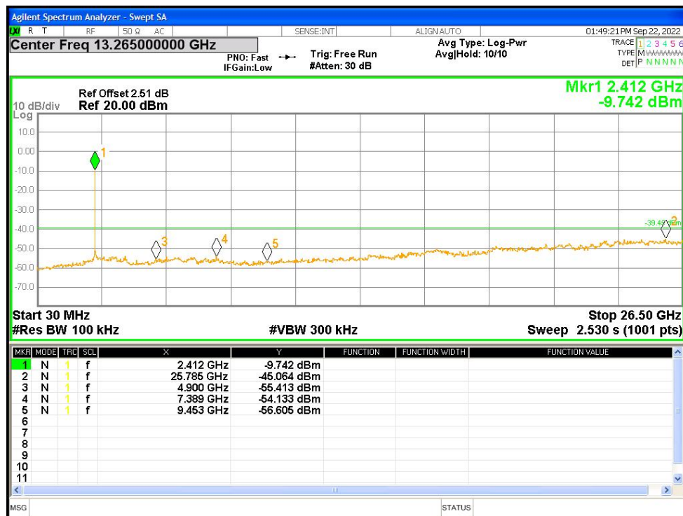
Tx. Spurious NVNT n20 2437MHz Ant1 Ref
