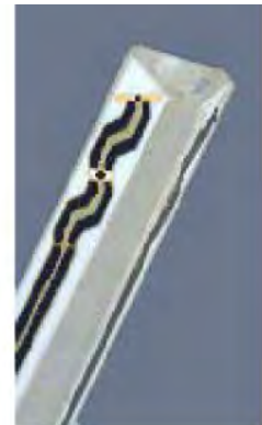
Figure 2.3 Probe Thick-Film Technique
