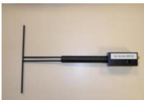
Figure 1 – Satimo COMOSAR Validation Dipole
