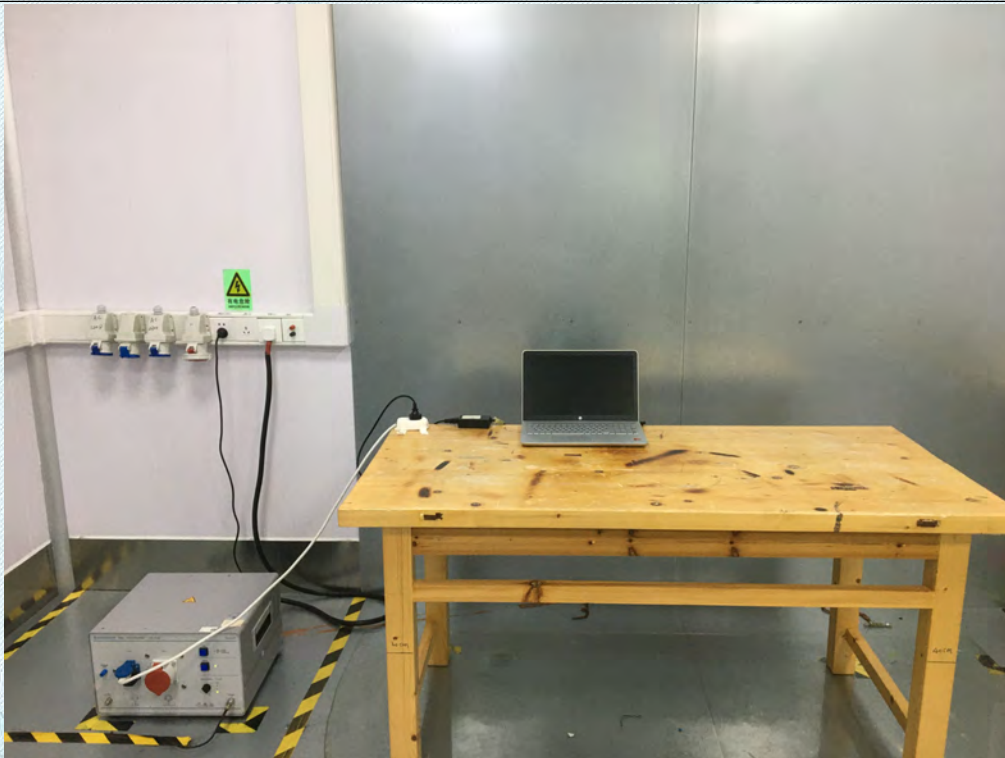
Conducted Emission at AC power line
