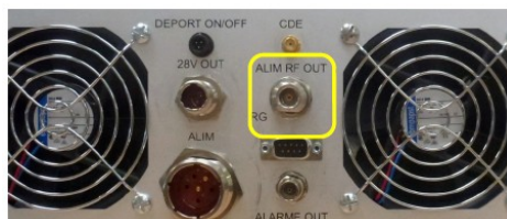
Inductive N connector Power supply output
