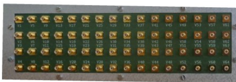
SMB connectors Analog \pm 5V Outputs
