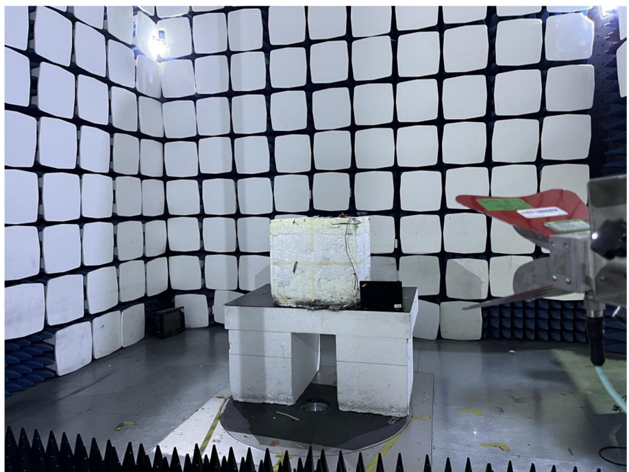
Radiation Emission Test Setup (1GHz to 18GHz)
