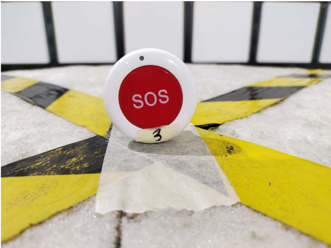
Radiated Emission Above 1GHz View
