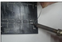
Clean up excess tin from IC pins
