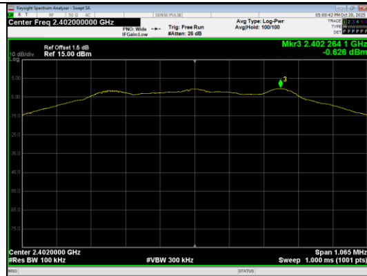
In-Band Reference Level BLE 1M_Channel 0
