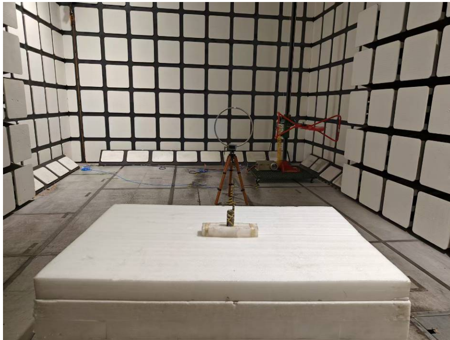
Radiated Emissions View (Below 30MHz)
