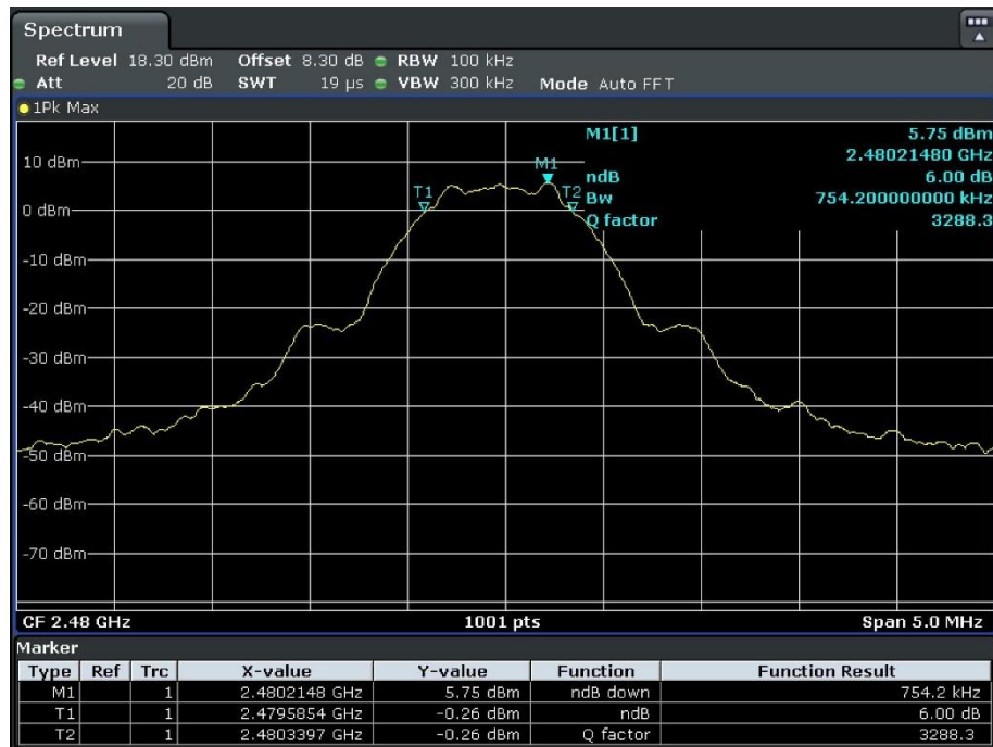
Figure 5. 6dB DTS Bandwidth: High Channel, 2480 MHz, BLE 1 Mbps Plot
