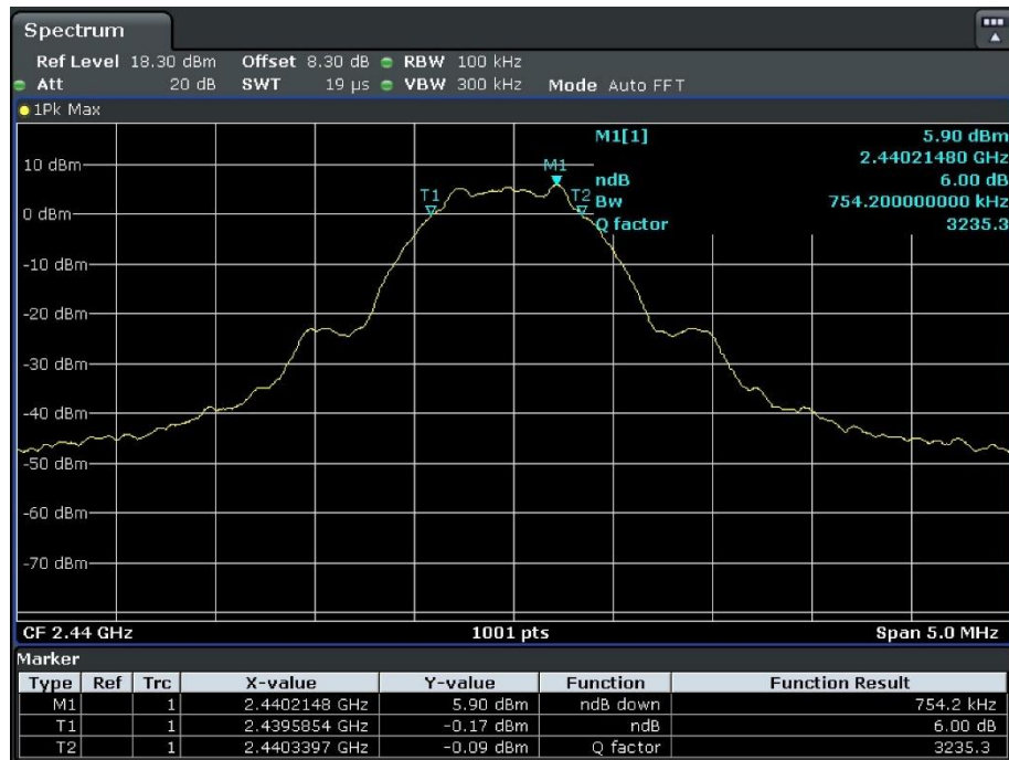
Figure 4. 6dB DTS Bandwidth: Mid Channel, 2440 MHz, BLE 1 Mbps Plot
