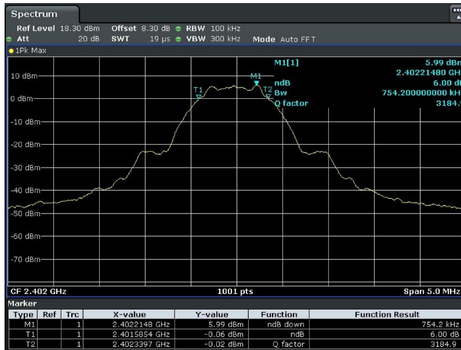
Figure 3. 6dB DTS Bandwidth: Low Channel, 2402 MHz, BLE 1 Mbps Plot
