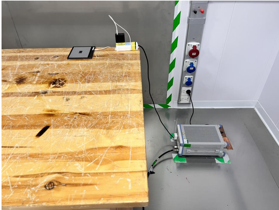
Conducted emission Test for DTS,NII
