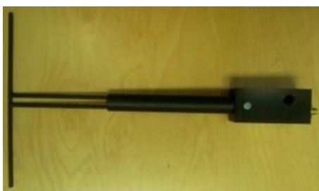
Figure 1 – MVG COMOSAR Validation Dipole
