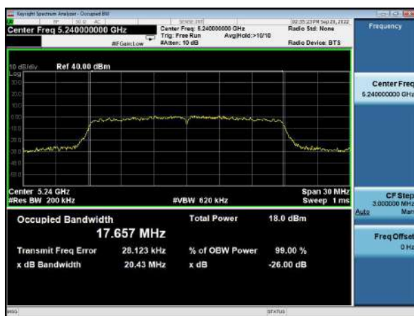
(802.11 n20) 26dB Bandwidth plot on channel 48
