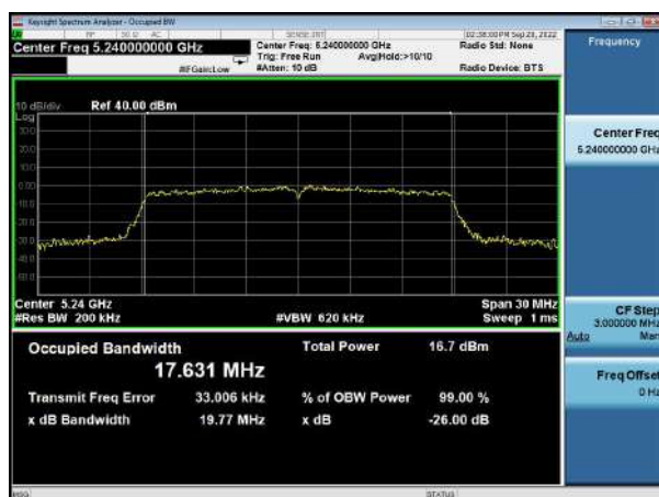
(802.11ac20) 26dB Bandwidth plot on channel 48
