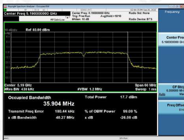
(802.11 n40) 26dB Bandwidth plot on channel 38
