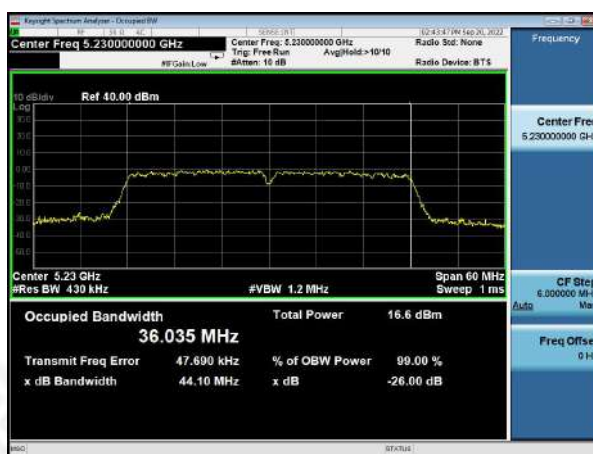
(802.11ax80) 26dB Bandwidth plot on channel 42
