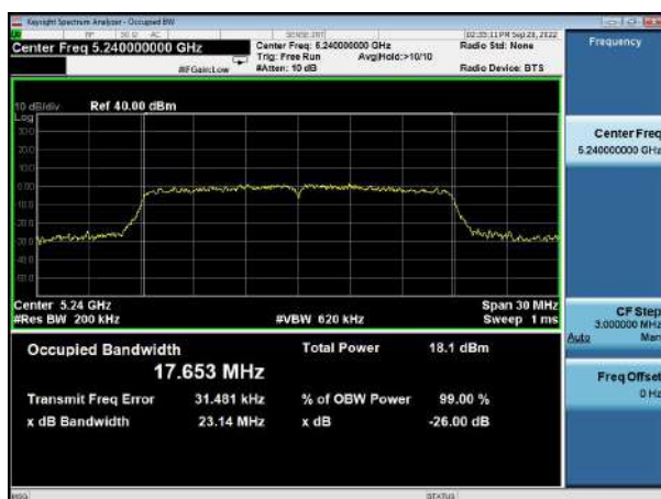
(802.11 n20) 26dB Bandwidth plot on channel 48
