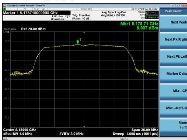
(802.11a20) PSD plot on channel 36
