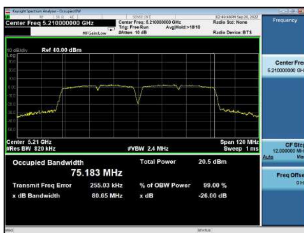
(802.11ac80) 26dB Bandwidth plot on channel 42
