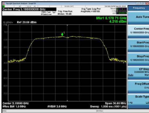
(802.11ac20) PSD plot on channel 40
