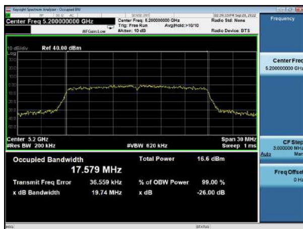
(802.11ax20) 26dB Bandwidth plot on channel 48
