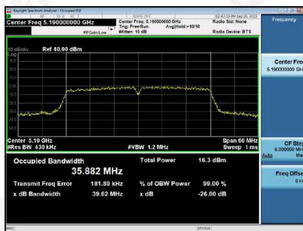
(802.11 ac40) 26dB Bandwidth plot on channel 42
