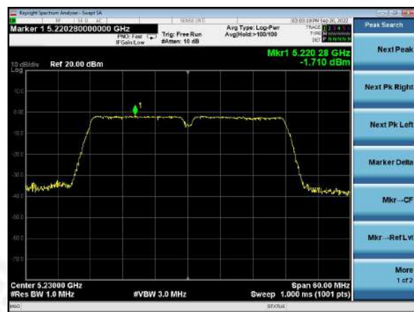
(802.11ac80) PSD plot on channel 42
