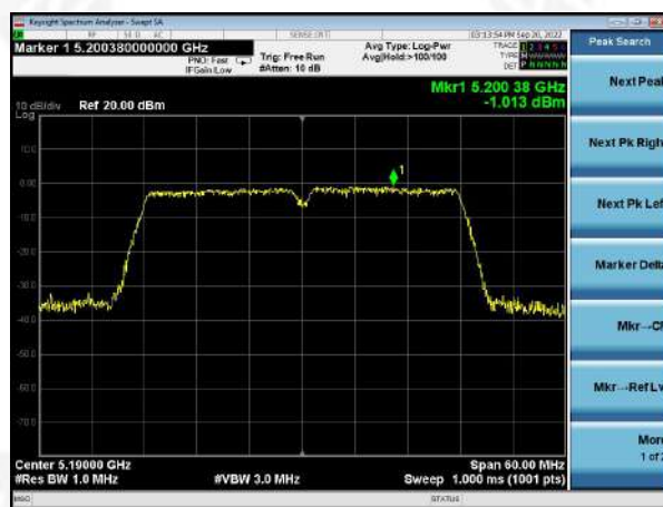
(802.11ac40) PSD plot on channel 46
