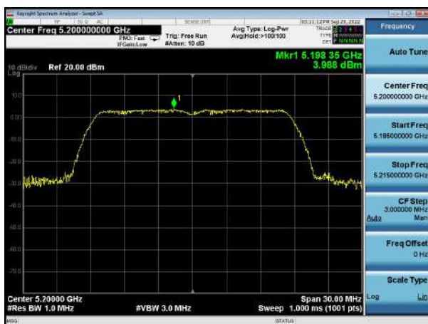
(802.11a20) PSD plot on channel 48
