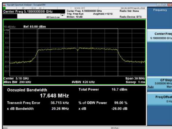
(802.11ac20) 26dB Bandwidth plot on channel 40
