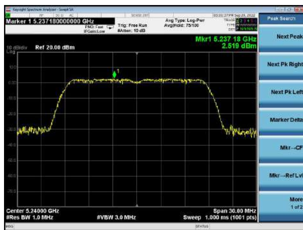
(802.11ax20) PSD plot on channel 48
