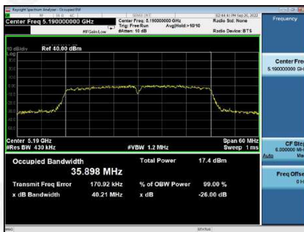
(802.11 ac40) 26dB Bandwidth plot on channel 42
