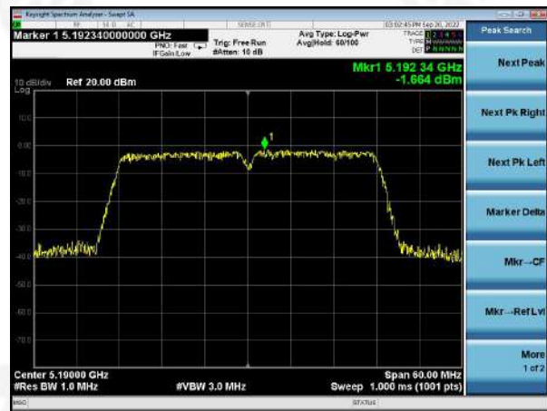
(802.11ac40) PSD plot on channel 46
