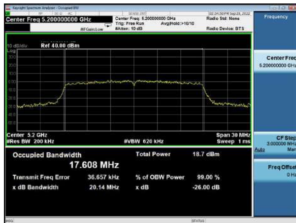
(802.11 n20) 26dB Bandwidth plot on channel 48
