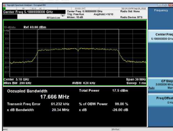
(802.11 n20) 26dB Bandwidth plot on channel 40
