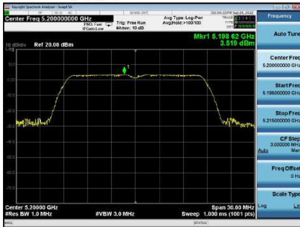
(802.11ax20) PSD plot on channel 40
