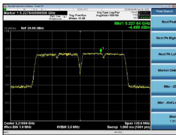
(802.11ac80) PSD plot on channel 42
