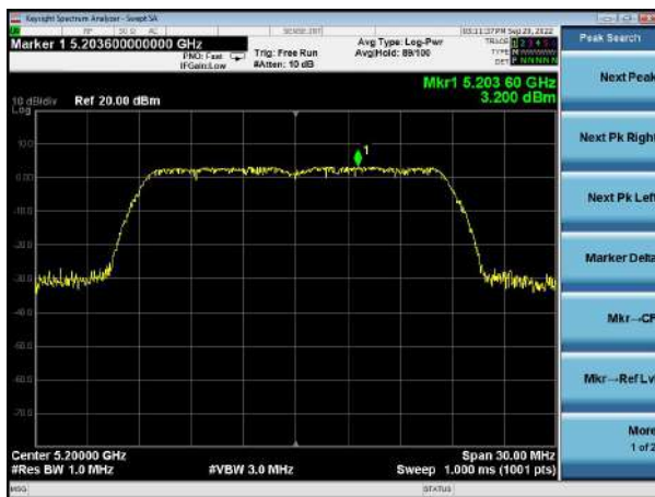
(802.11ac20) PSD plot on channel 48
