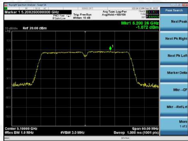
(802.11ax40) PSD plot on channel 46
