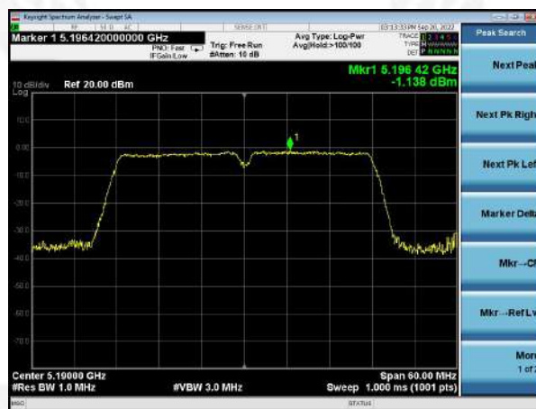
(802.11n40) PSD plot on channel 46
