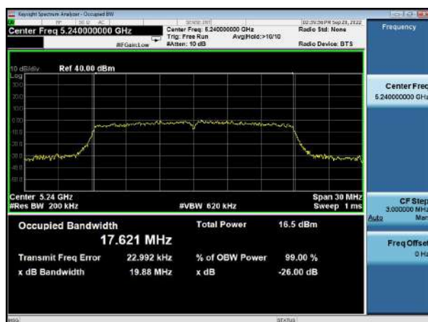
(802.11ax20) 26dB Bandwidth plot on channel 48
