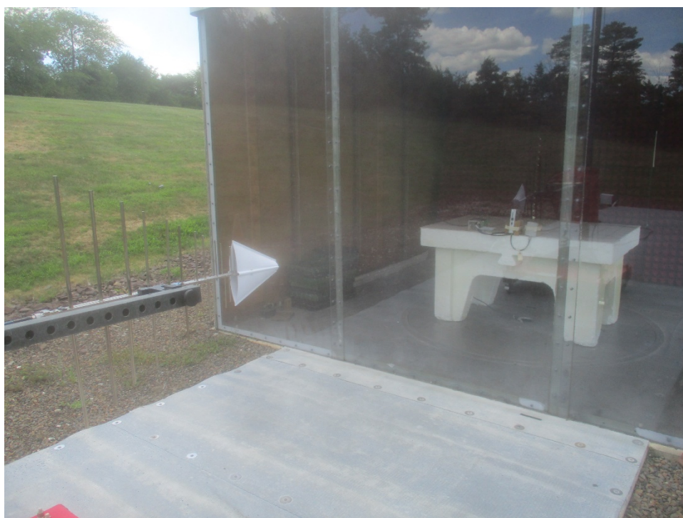
Vertical Antenna Polarization, 200 MHz to 1 GHz
