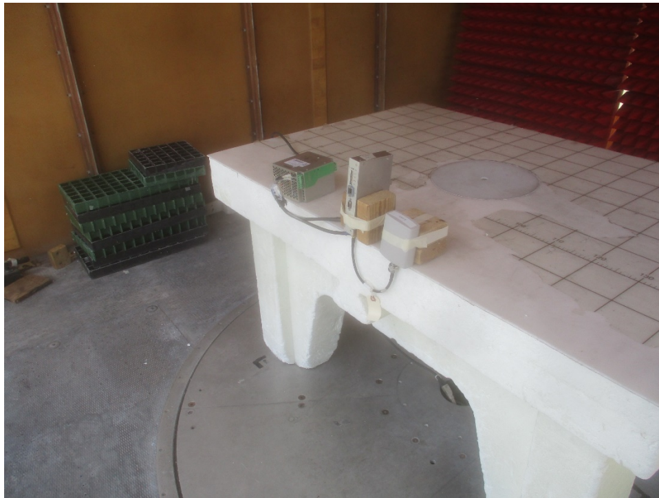
EUT Configuration, 30 MHz to 1 GHz
