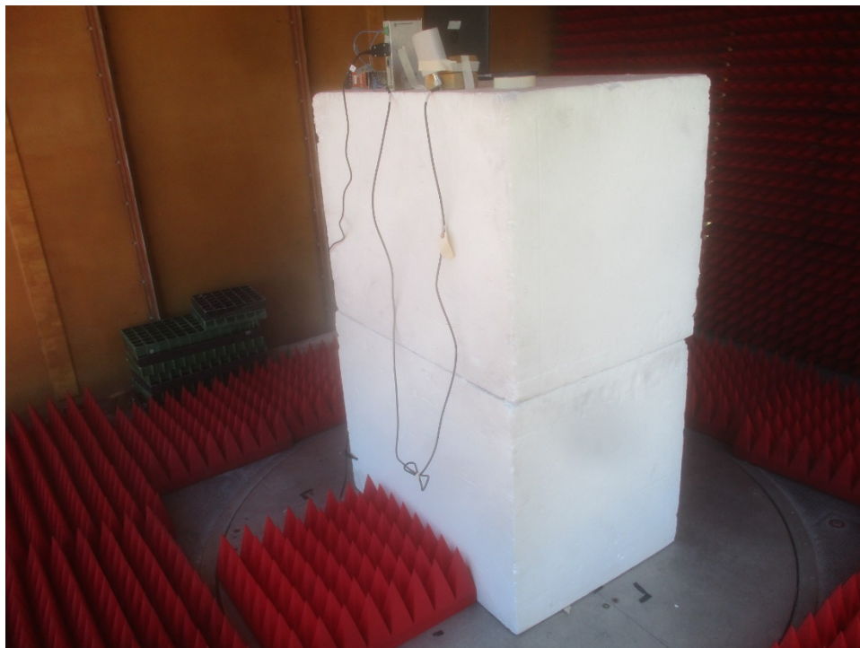
EUT Configuration, Above 1 GHz
