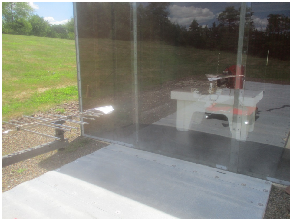
Horizontal Antenna Polarization, 200 MHz to 1 GHz
