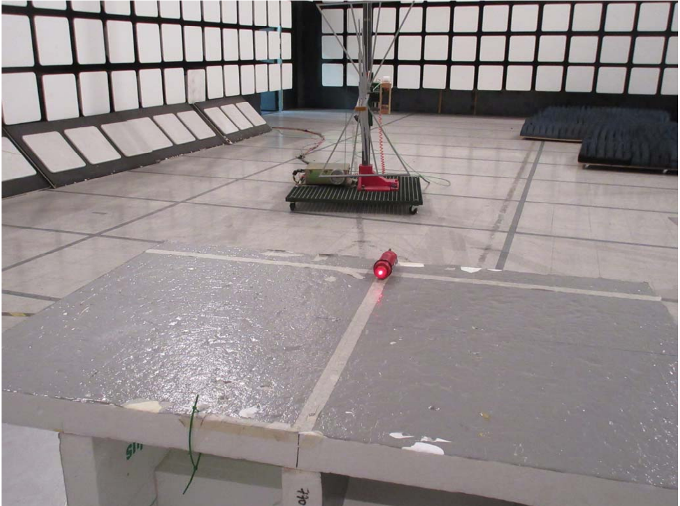
Radiated Emissions at 3 m EUT with 1.6 dBi Linx Technologies Inc ¼ wave whip, straight antenna, Orthogonal Position 1
