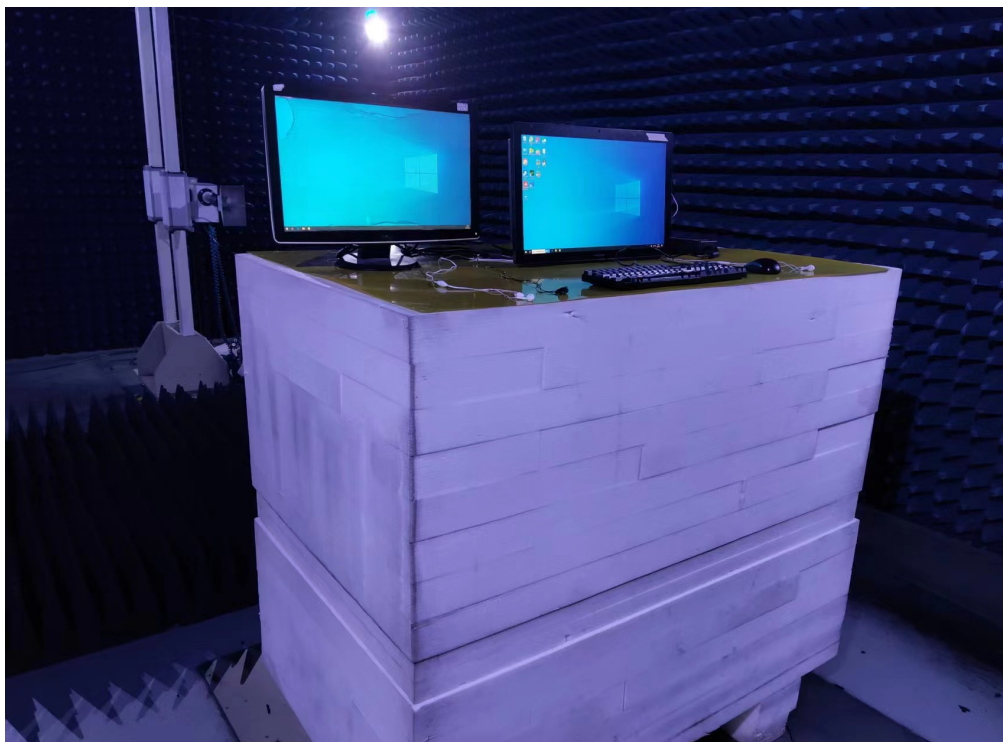
Photo of Radiated Emission Measurement (Above 1G)
