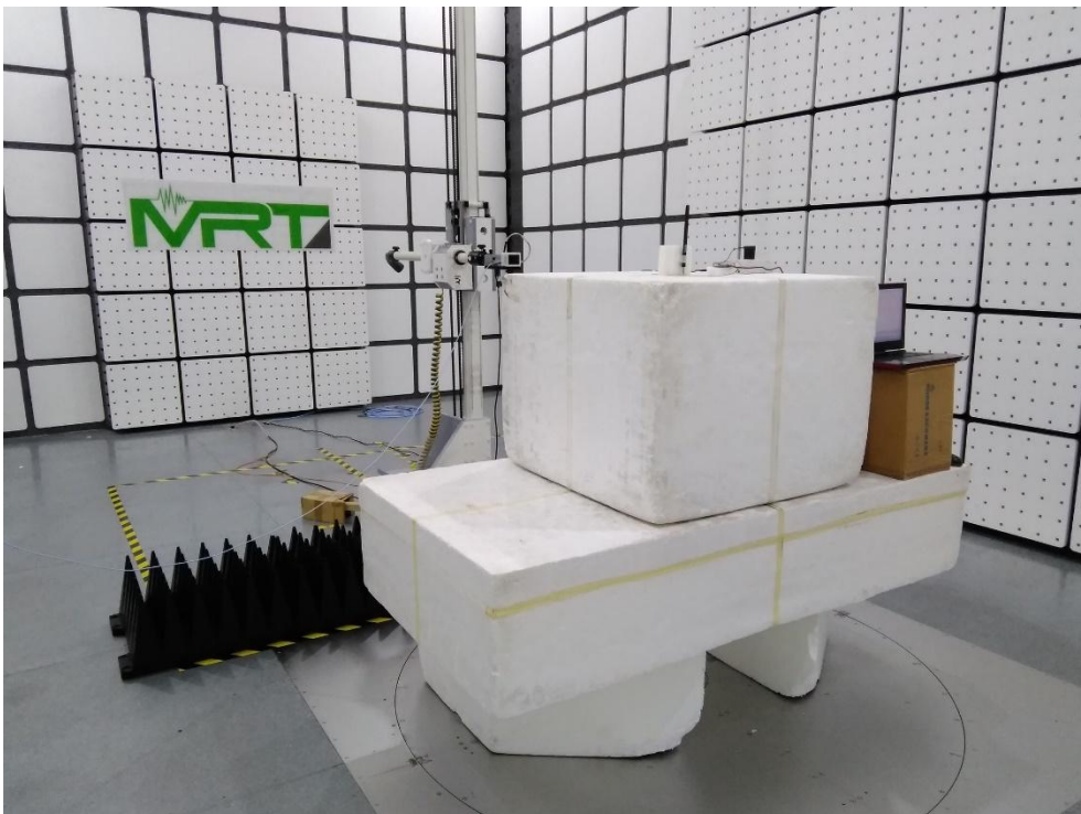
Description: Radiated Emission Test Setup for 18GHz~40GHz – GND Ant1
