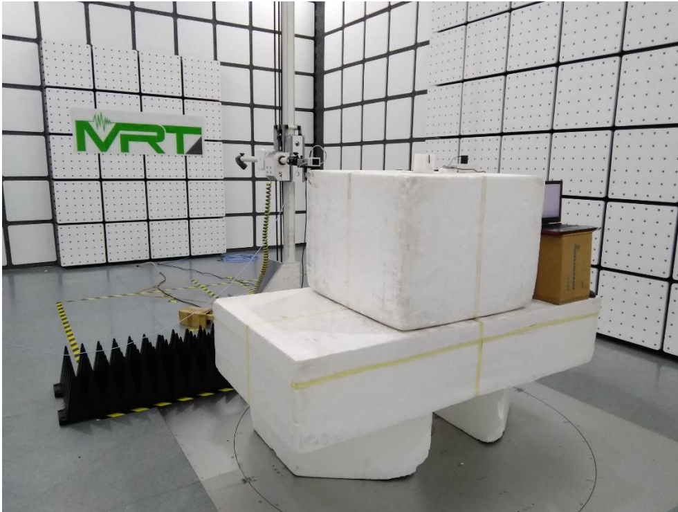
Description: Radiated Emission Test Setup for 18GHz~40GHz – GND Ant1
