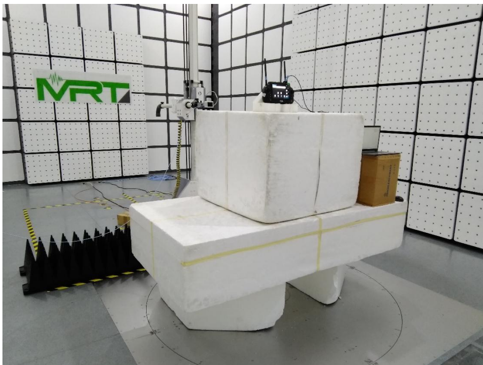
Description: Radiated Emission Test Setup for 18GHz~40GHz
