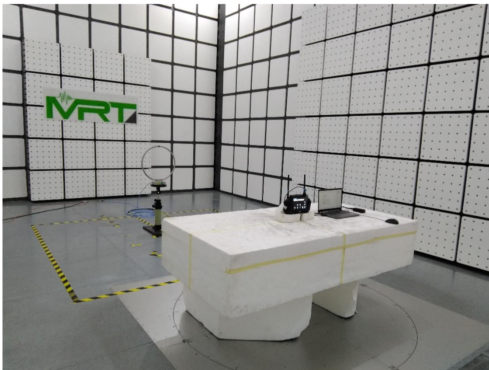
Description: Radiated Emission Test Setup for 18GHz~40GHz
