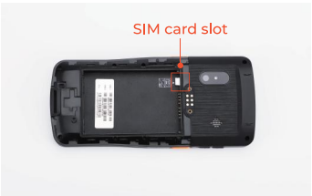
Figure 2- 2 the location of the card slot
