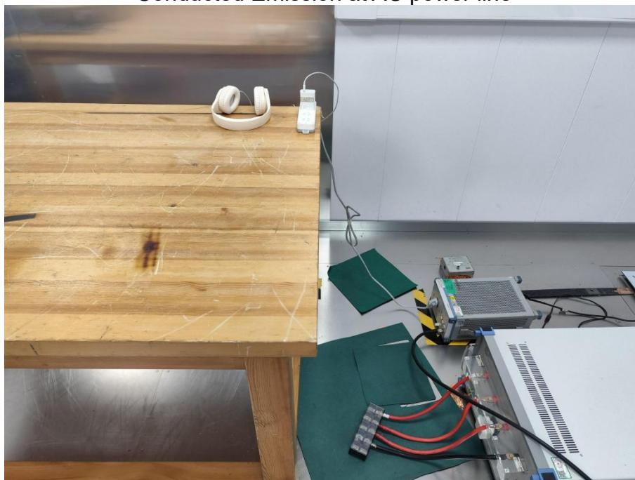
Conducted Emission at AC power line
