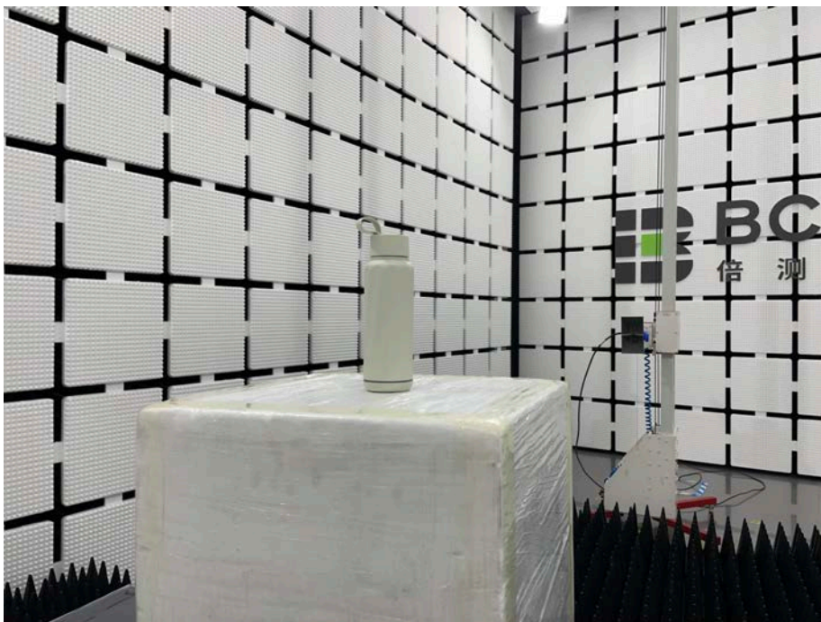
Spurious Emission Test Setup (Above 1GHz)
