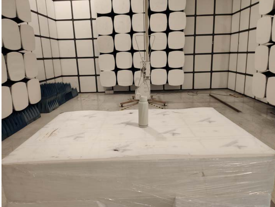
Spurious Emission Test Setup (Below 1GHz)
