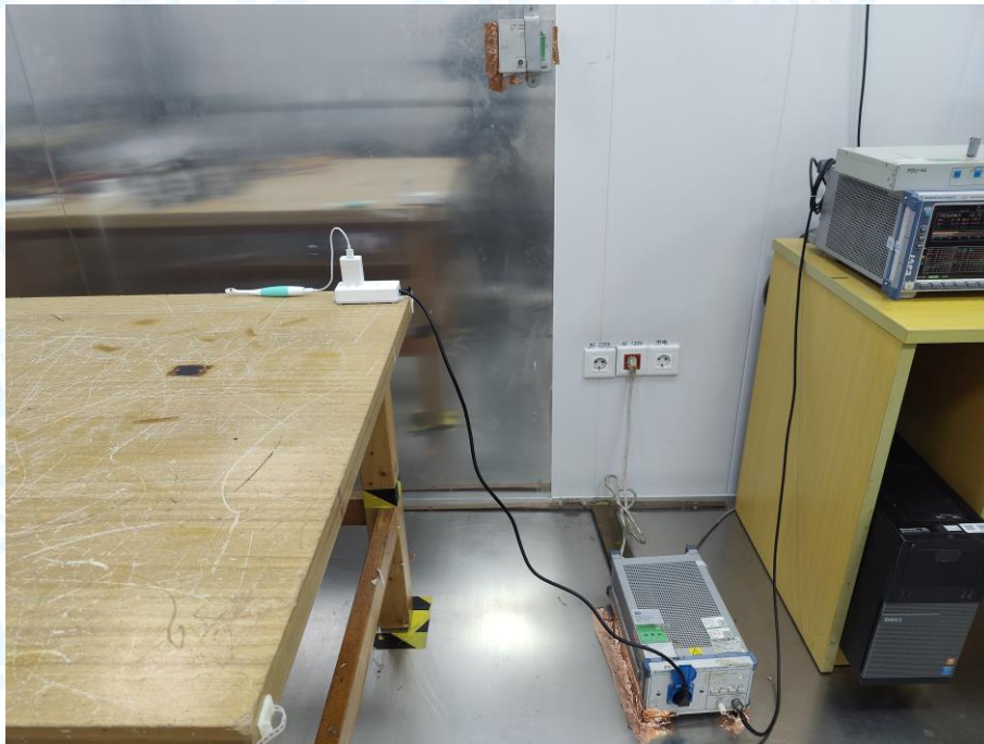
Photo of Setup for Conducted Emission
