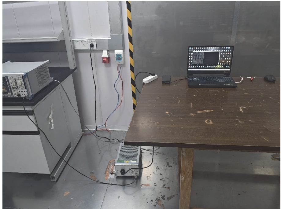
Conducted Emission Test Setup
