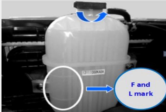
Front engine compartment: marking in coolant auxiliary tank
