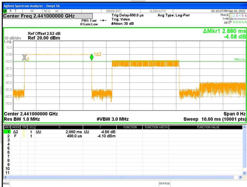
Dwell NVNT 1-DH5 2441MHz Ant1 Accumulated
