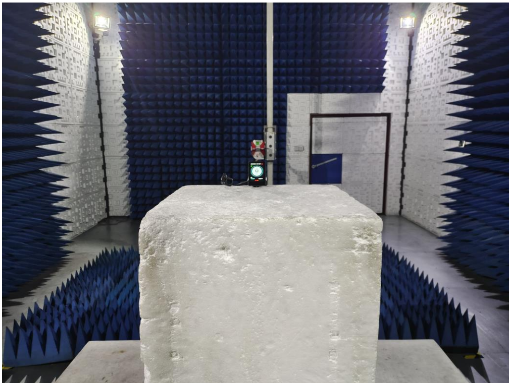
RADIATED EMISSION TEST SETUP ABOVE 1GHz
