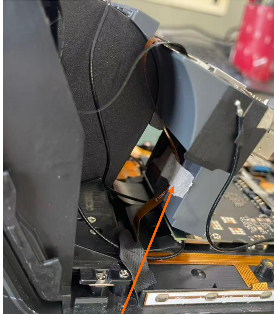
Secure the ribbon cable with masking tape
