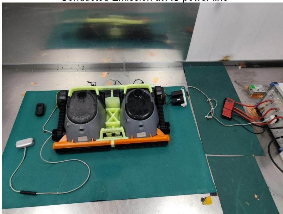
Conducted Emission at AC power line
