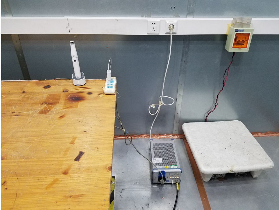
Picture 2 Conducted Emission Test Setup
